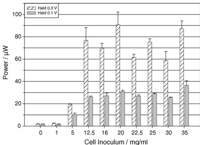
Fig. 3. Electrical power generated as a function of concentration of yeast inoculum at 30 °C and 0.1 M glucose. Cell voltage was stepped from OCV to 0.3 V for 5 min, and then stepped to 0.1 V for 5 min. Average current at the end of 5 min was used to calculate power.
