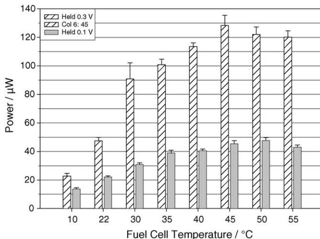
Fig. 5. Power generated as a function of cell temperature.
