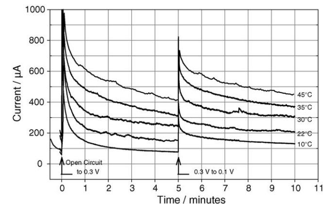
Fig. 4. Electrical current produced as a function of temperature with 20 mg ml<sup>-1</sup> of yeast inoculum and 0.1 M glucose. Cell voltage was stepped from OCV to 0.3 V for 5 min, and then stepped to 0.1 V for 5 min.
