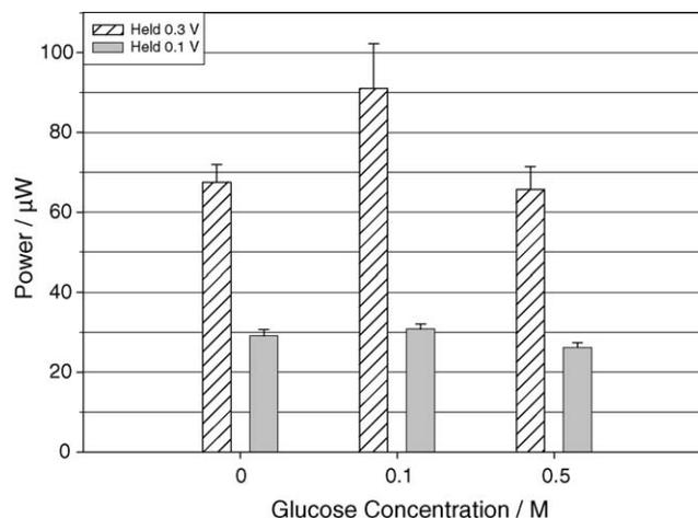
Fig. 6. Power generated as a function of glucose concentration for 20 mg ml<sup>-1</sup> yeast inoculum at 30 °C.
