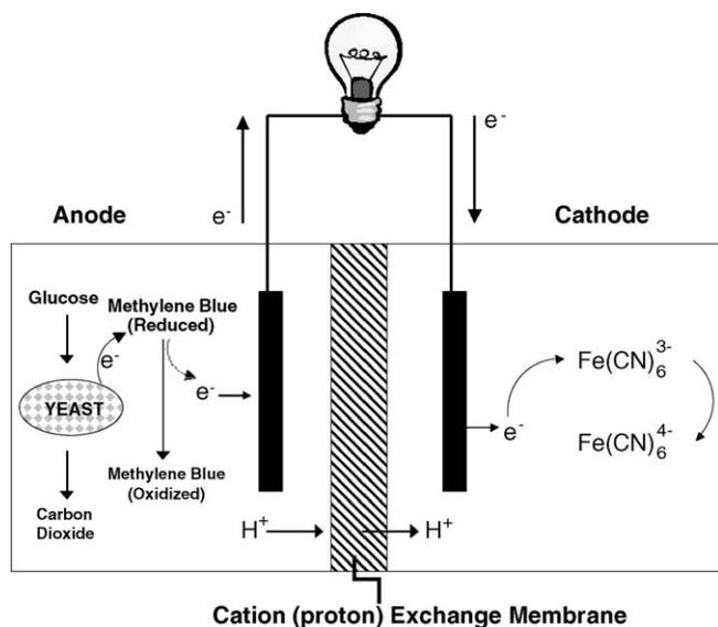
Fig. 2. Schematic of the biological fuel cell system.
