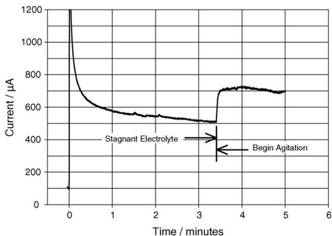
Fig. 7. Effect of solution agitation at 45 °C and 0.1 M glucose with 20 mg ml<sup>-1</sup> yeast inoculum held at 0.3 V.
