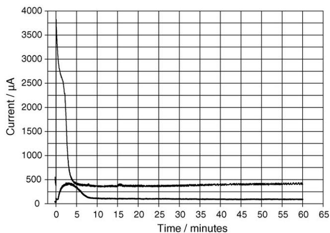
Fig. 8. Comparison of the effect of oxygen-saturated (lower trace) and anoxic (upper trace) solutions on current at 45 °C and 0.1 M glucose with 20 mg ml<sup>-1</sup> yeast inoculum held at 0.3 V for 1 h.
