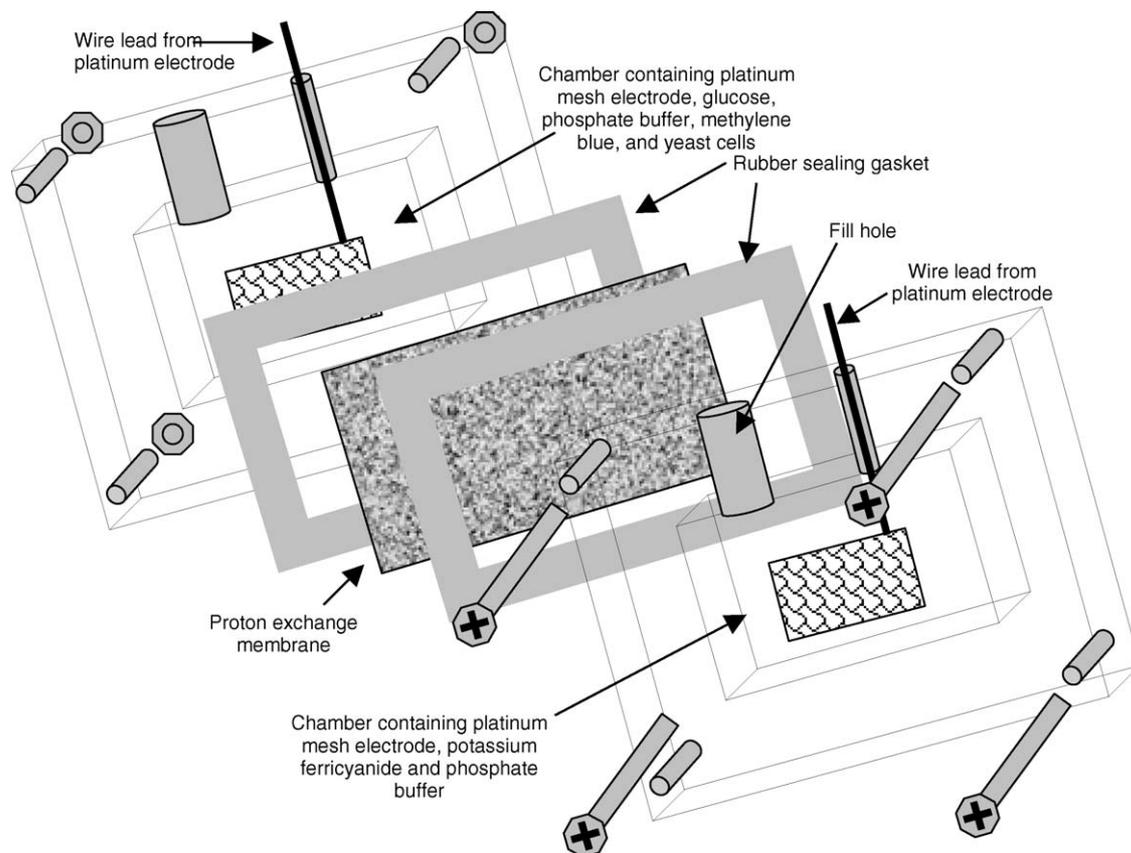
Fig. 1. Construction diagram of the plexiglass fuel cell.
